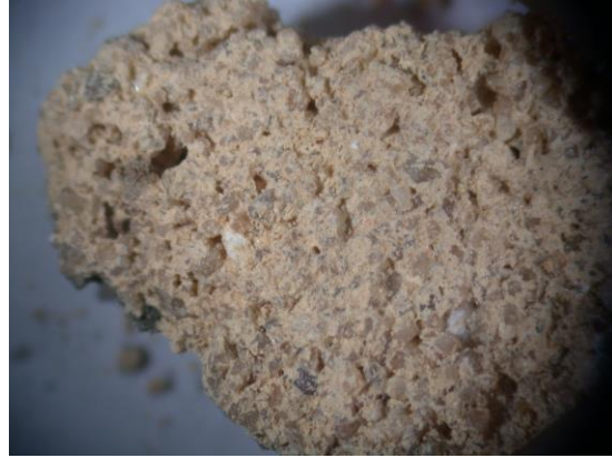
Photomicrograph of core of brick bedding mortar – based on lime and sand with clay and possibly brick dust (incident color-balanced light @ 10x magnification).
