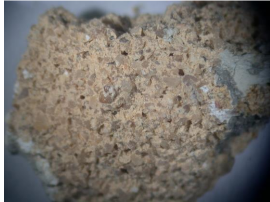
Photomicrograph of core of brick bedding mortar (incident color-balanced light @ 10x magnification). White binding material attached at either side of this fragment does not appear to be part of the matrix.
